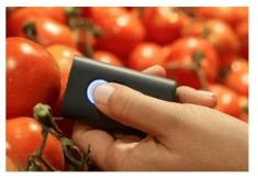
near-infrared (NIR) spectroscopy to scan physical materials. In just a few moments, the device can compare a scanned object to a database of physical objects to see if the subject fits within a signature of previously identified objects.
